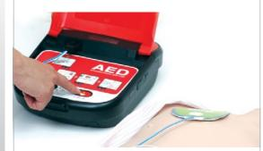
**3. PUSH THE SHOCK BUTTON.** Set the mode to adult or paediatric, then wait for the shock button to flash 'ready' for shock delivery. 1 COVER Protected icon sheet, shock button, Adult/Paediatric mode switch.
